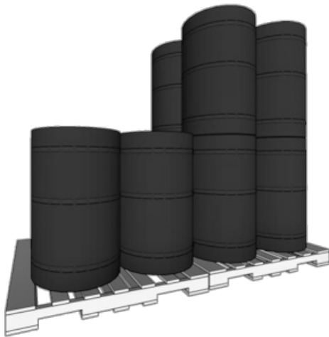
Cylinders Stored Upright
